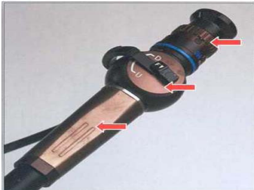
Cosmetic damage to an ENF-P3 rhinolaryngoscope. The black anodized coating on various parts of the control section has been removed, resulting in a silvery and/or golden tinge. Similar loss of anodization is usually observed on portions of the light guide connector.
