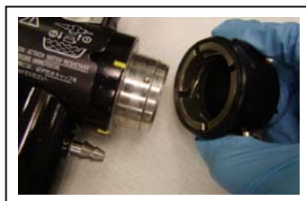
Fig. 2. Water resistant cap removal from Olympus videoscopes
